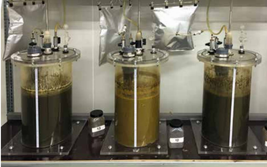
Panta Rhei – everything flows – feedstock example from 90% chicken manure at 7.8 g NH 4 + and 90 g/l oDM – in lab reactors at ISF Schaumann Research
